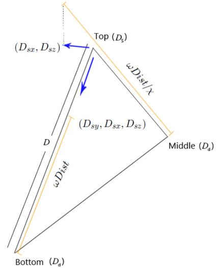
Figure 3: The deformation coordinates of a single triangle.
