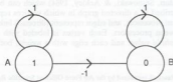
FIGURE 1. A Boltzmann machine for n = 1 with two processors, labelled "A" and "B." I = \{A\} , O_n = \{B\} and A_n = \{\} .
