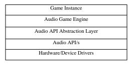
Figure 1. Layered Software Architecture.
